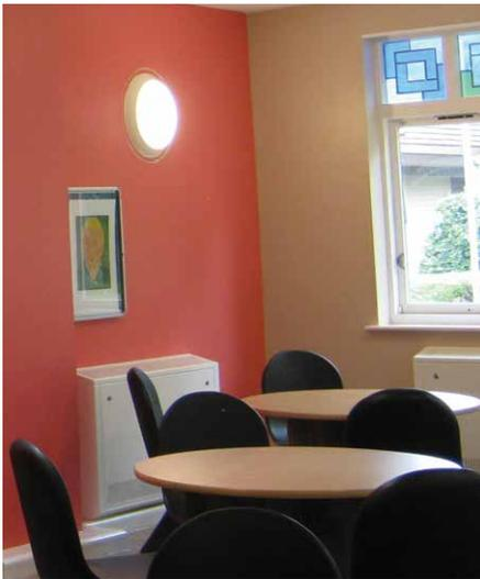
Designplan Lighting were appointed to design and commission a lighting system in all corridors, day areas, TV rooms and dining rooms. Adjustable light levels and colour temperatures were incorporated to aid rest and recuperation. Existing lighting points and cabling were used for minimal disturbance to service users.
