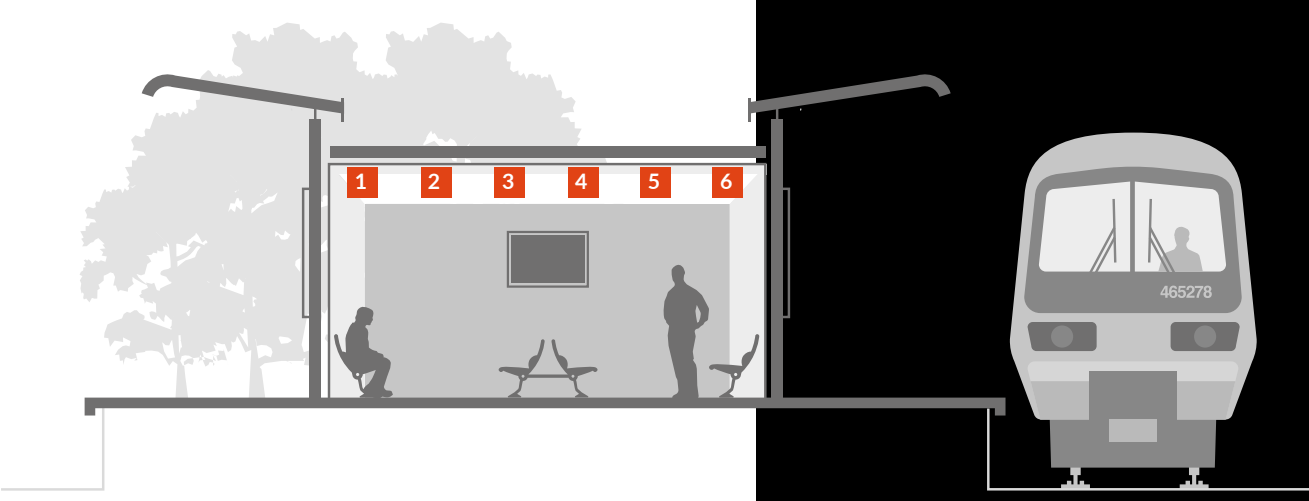
6 DL86 IP65 IK11 (50J) Provides a consistent light distribution.
